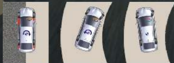
Braking control on a road surface with different left and right side traction characteristics
