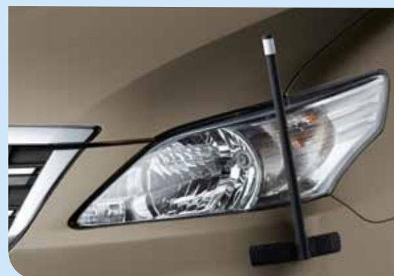
Fender Pole PZ058-OK601 It helps the driver in judging the far edge of the car and helps in better manoeuvring.
